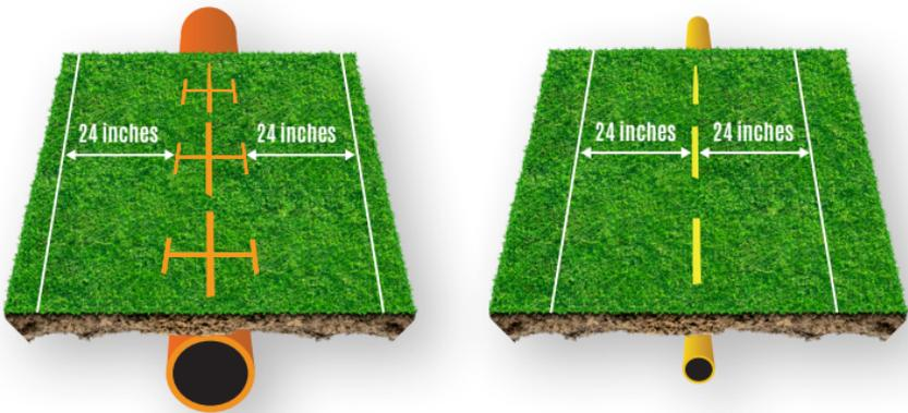
**NOTE:** Location markings are approximate, and the exact location may vary by up to 24-inches for gas, electric, communications, and most wastewater and potable water. (See KSA 66-1802)
